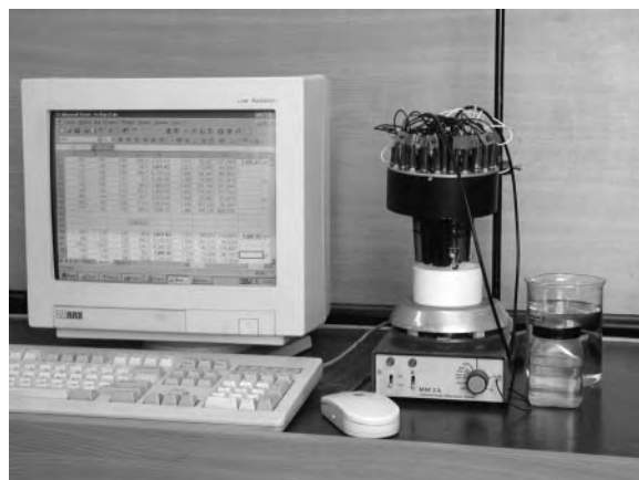
Figure 2. A photograph of a laboratory prototype of the electronic tongue based of potentiometric chemical sensors. 32
